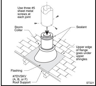
Fig. 34 Roof support and flashing.
